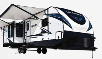
**UVW** (Unloaded Vehicle Weight) is the typical weight of the unit as manufactured at the factory. It includes all weight at the unit's axle(s) and tongue or pin and LP Gas. The UVW does not include cargo, fresh potable water, additional optional equipment or dealer installed accessories. \*Estimated Average based on standard build optional equipment.
